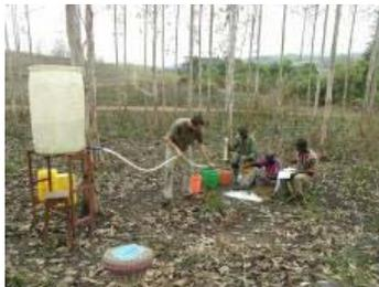
Figure 4. Experimental design for the artificial rainfall simulations.
