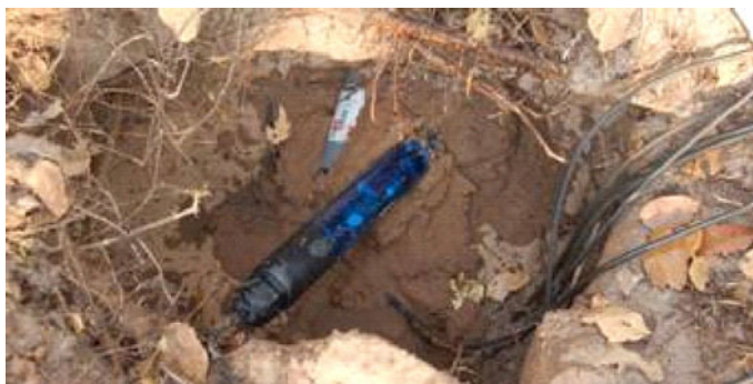
Figure 10. A tensiometer for soil water potential measurements.
