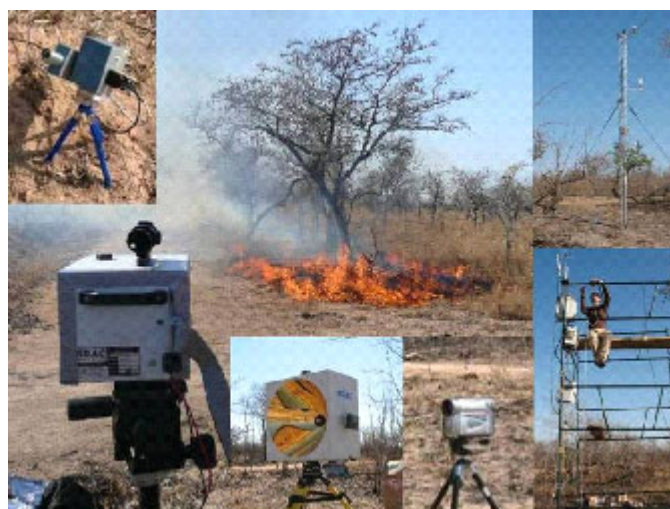
Figure 9: the different sensors utilised during the fire experiment, in order to measure the gas emissions, the fire spread, the fire radiative energy, the fuel consumption, and the smoke and the particles production, and estimate the burnt biomass.
