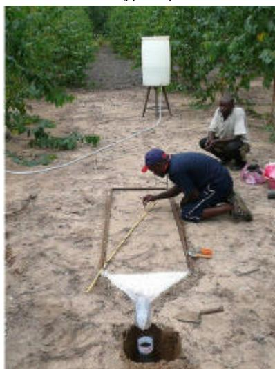
Figure 5 - The manual rainfall simulator built in Congo.
